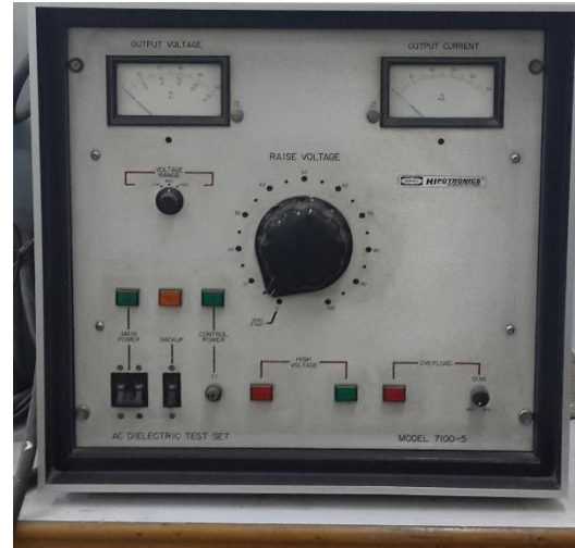
High voltage AC (HVAC) source
