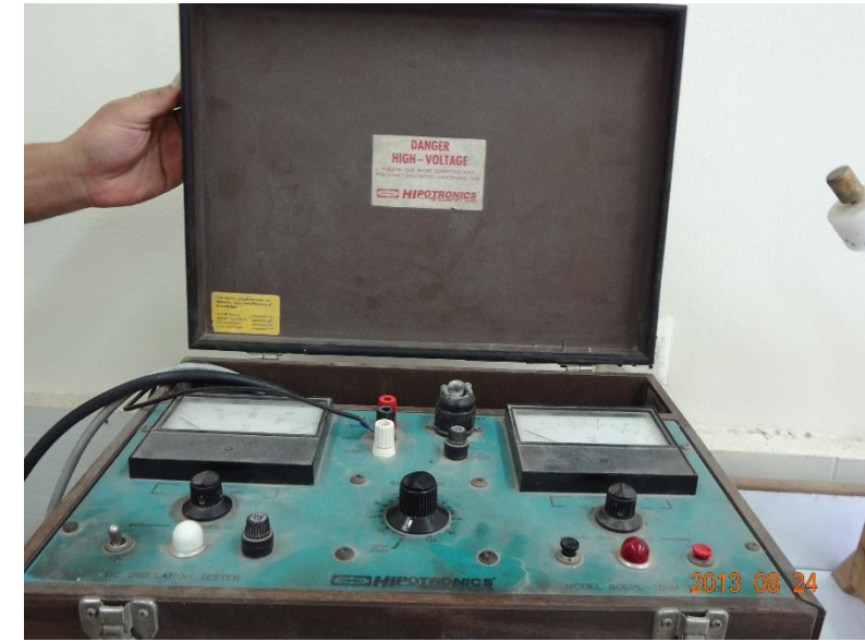
High voltage DC (HVDC) source
